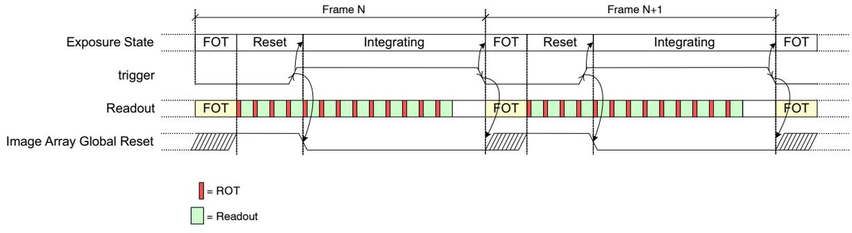
Figure 25. Exposure Time Control in Global-Slave Mode
