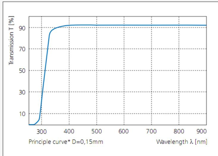
Figure 51. Transmission Characteristics of Glass Lid
