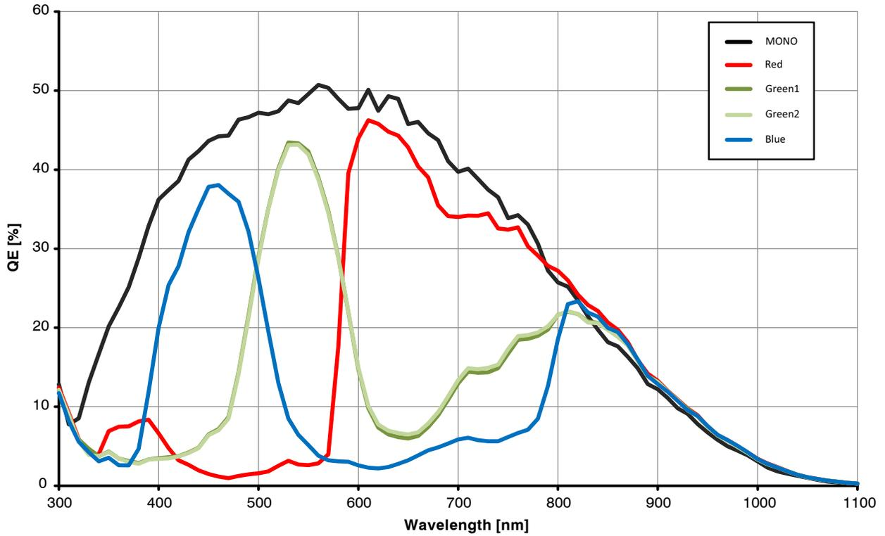
Figure 3. Quantum Efficiency Curve for Mono and Color
