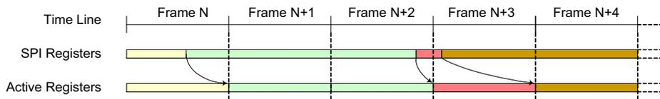
**Figure 19. Frame Synchronization of Configurations (no freezing)**
