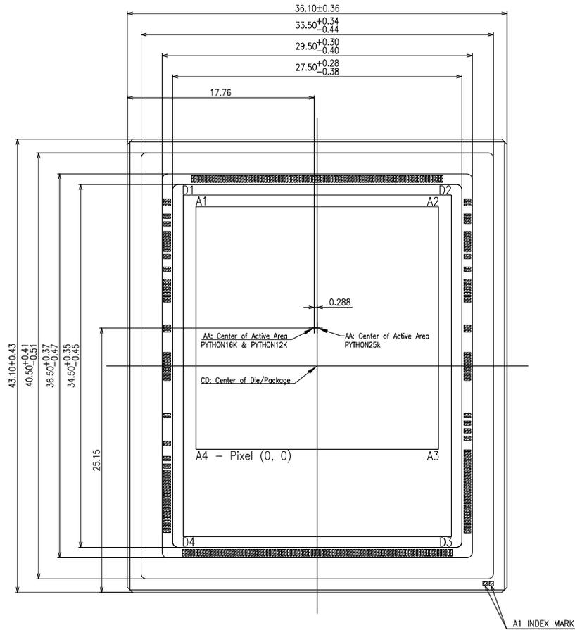
**Figure 50. Graphical Representation of the Optical Center**
