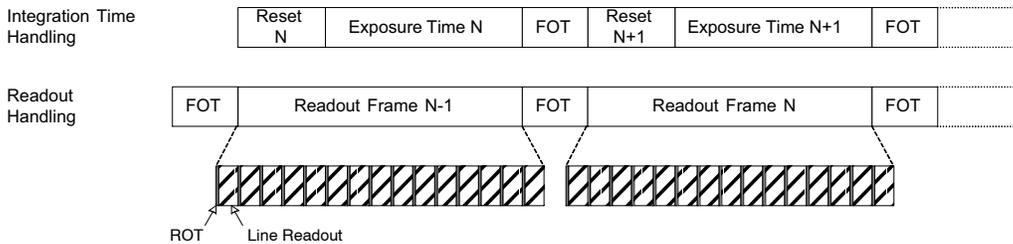
Figure 11. Pipelined Shutter Operation in Master Mode
