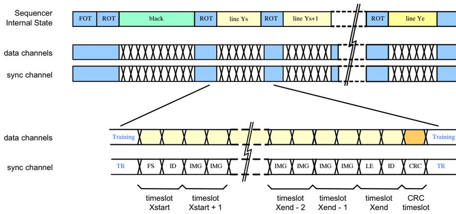
**Figure 32. Timeline for Single Window Readout**
