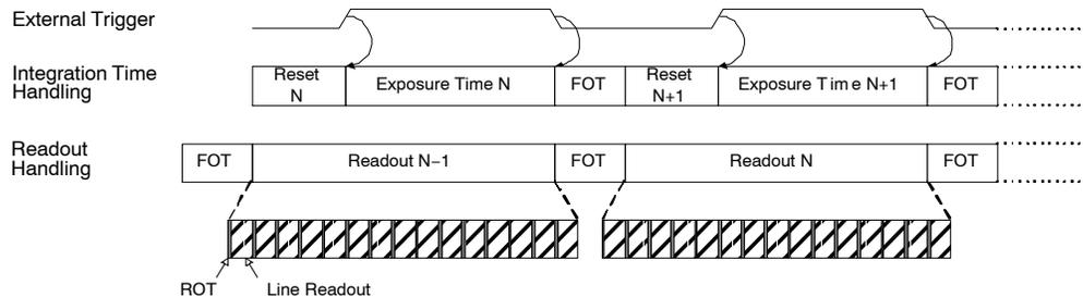
Figure 12. Pipelined Shutter Operation in Slave Mode
