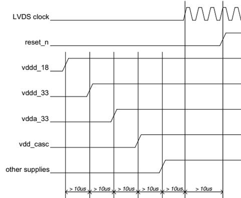
Figure 17. Power-up Procedure
