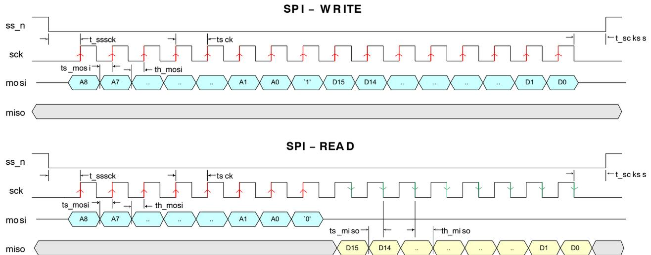
**Figure 21. SPI Read and Write Timing Diagram**
