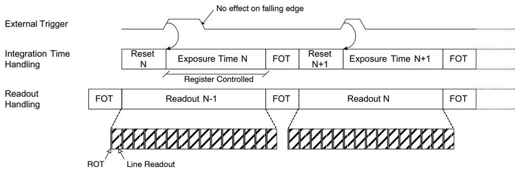
**Figure 13. Triggered Shutter Operation in Master Mode**
