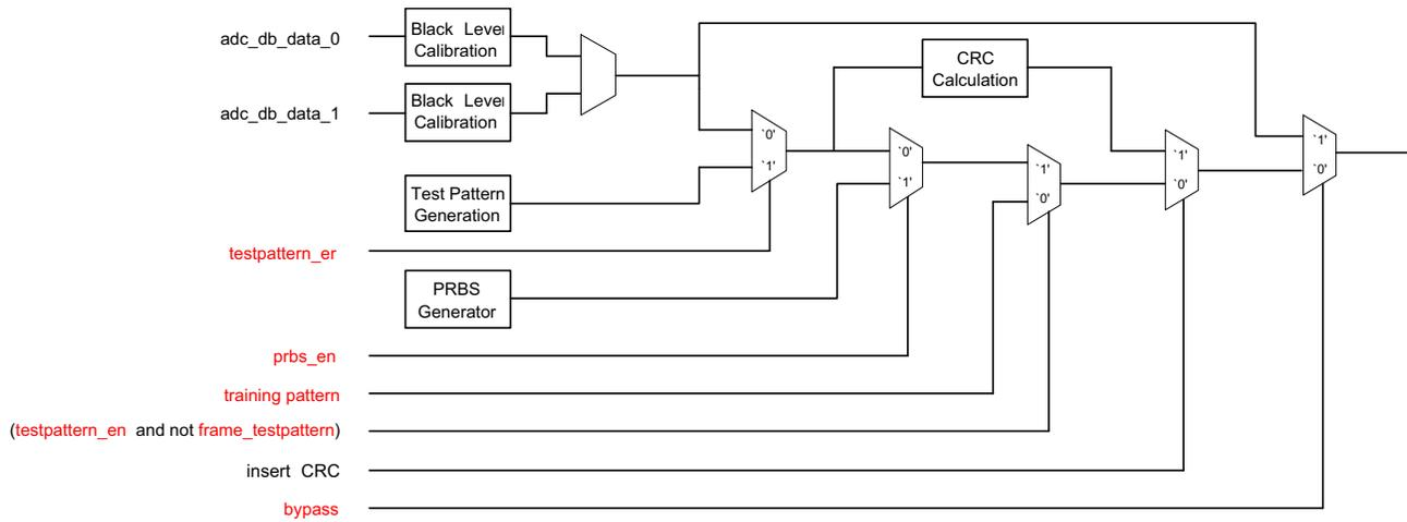
**Figure 48. Functional Block Diagrams for the Data Channels**
