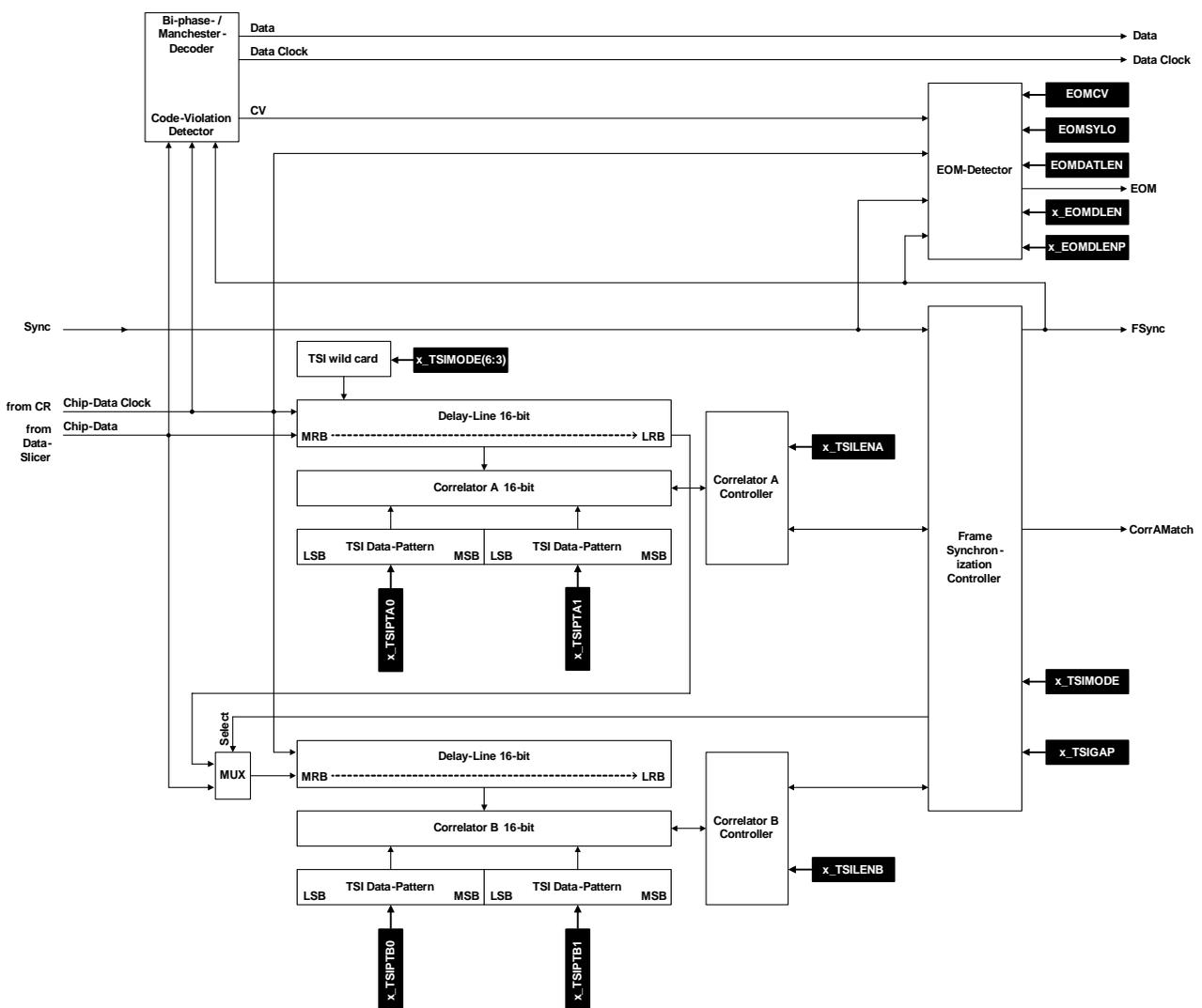
**Figure 26** Frame Synchronization Unit
