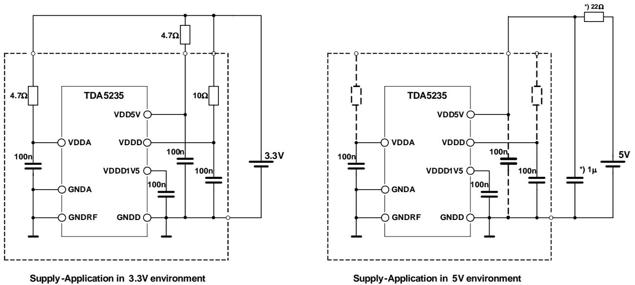
\*) When operating in a 5V environment, the voltage-drop across the voltage regulators 5 → 3.3V has to be limited, to keep the regulators in a safe operating range. Resistive or capacitive loads (in excess to the scheme shown above) on pins VDDA and VDDD are not recommended.
