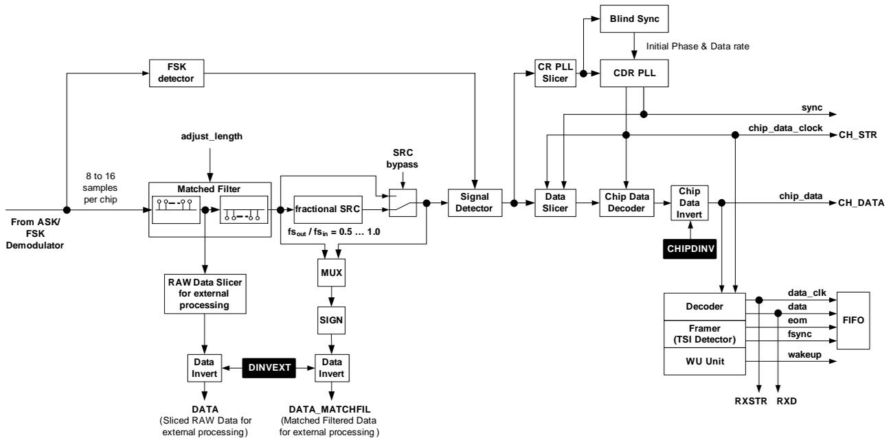
**Figure 15 Functional Block Diagram Digital Baseband Receiver**
