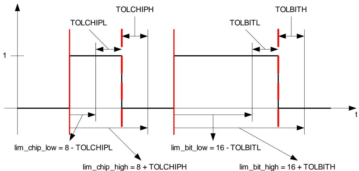
**Figure 21 Definition of Tolerance Windows for the CDR**
