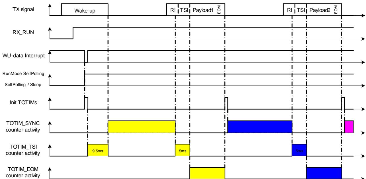
**Figure 75** TOTIM Behavior without Presence of Interferer
