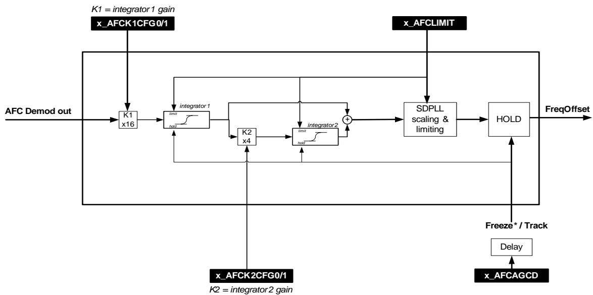
**Figure 11 AFC Loop Filter (I-PI Filtering and Mapping)**
