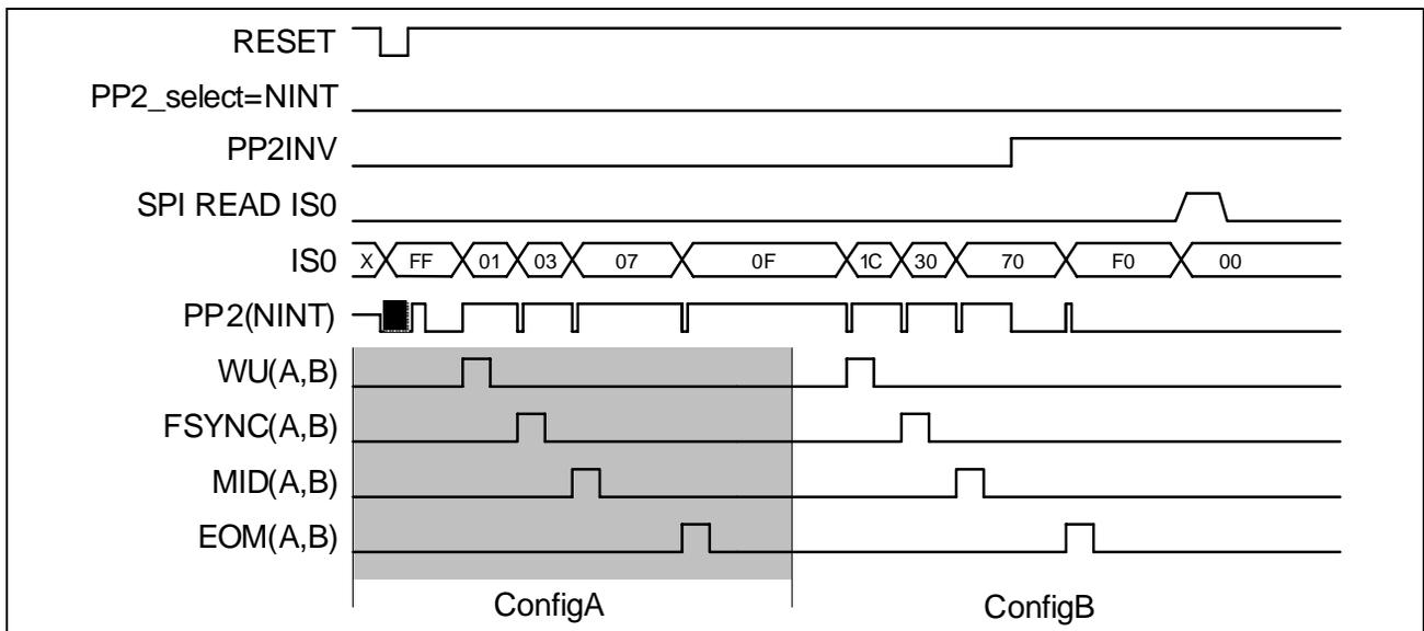
Figure 57 Interrupt Generation Waveform (Example for Configuration A+B)
