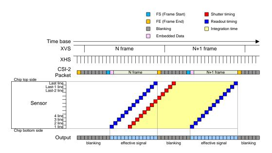
Image Drawing of Shutter Operation
