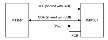
Pin connection of serial communication
