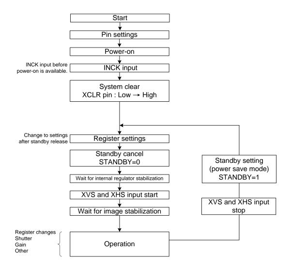
Sensor Setting Flow (Sensor Slave Mode)
