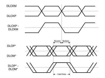
(Output load capacitance: 8 pF)
