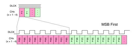
Example of Data format in low-voltage LVDS serial 10-bit output
