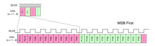
Example of Data format in low-voltage LVDS serial 12-bit output
