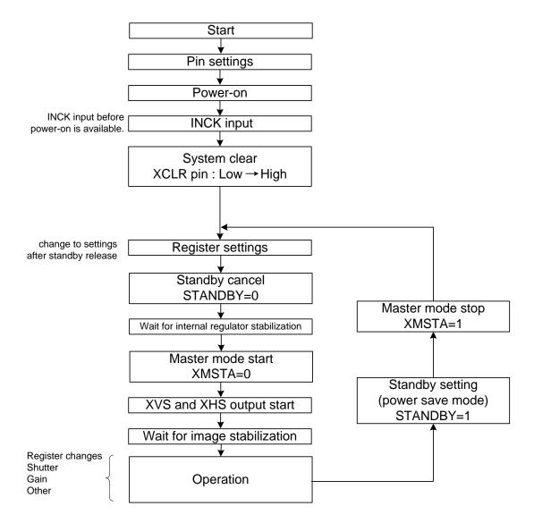
Sensor Setting Flow (Sensor Master Mode)
