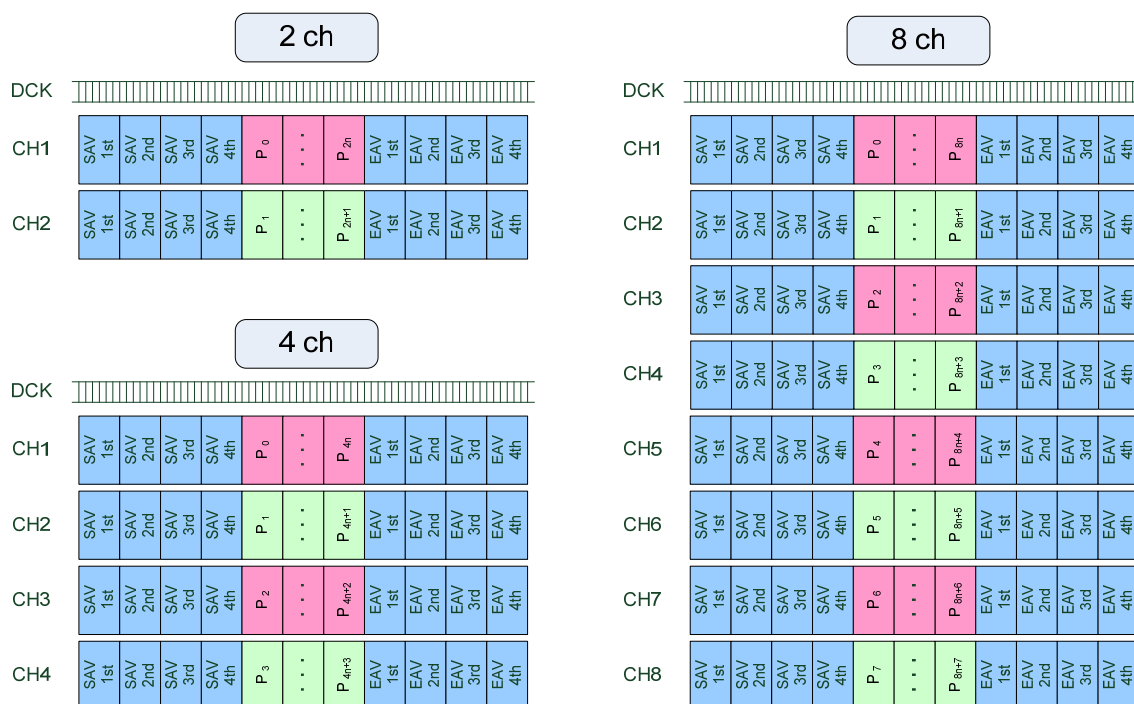
Output Format of Low voltage LVDS Serial 2 ch / 4 ch / 8 ch
